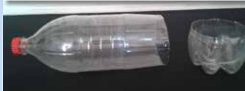
**2** USING THE MEASURING CUP, POUR 10 ML OF WATER INTO THE TOP PART OF THE BOTTLE AND MARK THE LEVEL OF THE WATER. ADD ANOTHER 10 ML AND MARK THE NEW LEVEL AGAIN, AND REPEAT THIS UNTIL YOU HAVE A FEW MARKINGS UP THE BOTTLE. THEN EMPTY THE BOTTLE.
