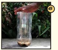
Find a stable, open place to leave your rain gauge and remember to check it after rain! Throw out the rainwater after you have measured it, so your gauge is ready for the next rainfall.
