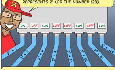
BY TURNING ON DIFFERENT WIRES (WHICH IS LIKE ADDING UP THE DIFFERENT CARDS), COMPUTERS CAN MAKE ANY NUMBER WE WANT!
