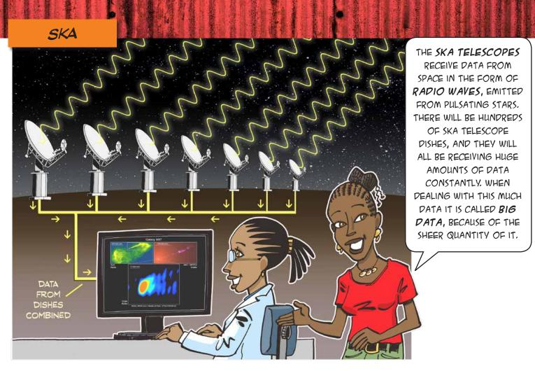
Various Functions then need to be performed, such as removing the interference, calibrating all of the data and finally turning it into an image that we can see (like the MeerKAT First Light image). Normal computers aren't powerful enough to do this; in fact, it would take 100 million normal computers to do all of this! For this reason, the SKA will need to use supercomputers.
